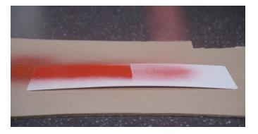
When dry, any residue can simply be wiped off or removed with low pressure water spray. Since the coating prevents paint and inks from adhering, a tagger will quickly find his efforts useless and give up.
